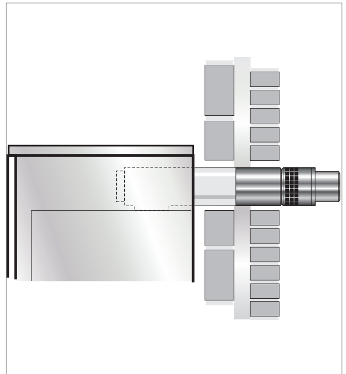
Figure 9-9: Low level balanced flue
