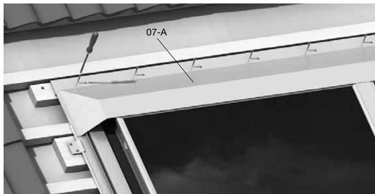
**Figure 73:** Fixing left hand Top Cover Flashing (07-A)
