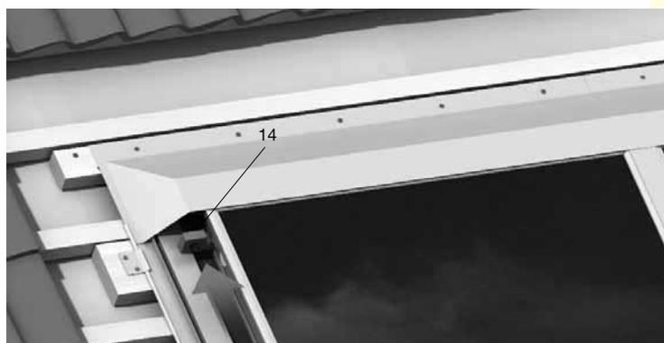
**Figure 74:** Fitting Foam Block (14)
