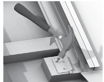
**Figure 63:** Securing Side Gutter Clips
