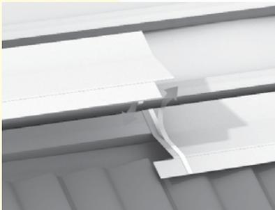
**Figure 55:** Installation of Additional Bottom Flashings
