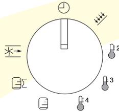
Figure 3-2: Display selector switch
