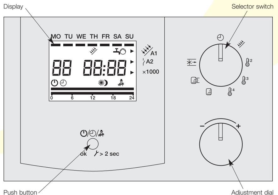
**Figure 3-1:** Controller features
