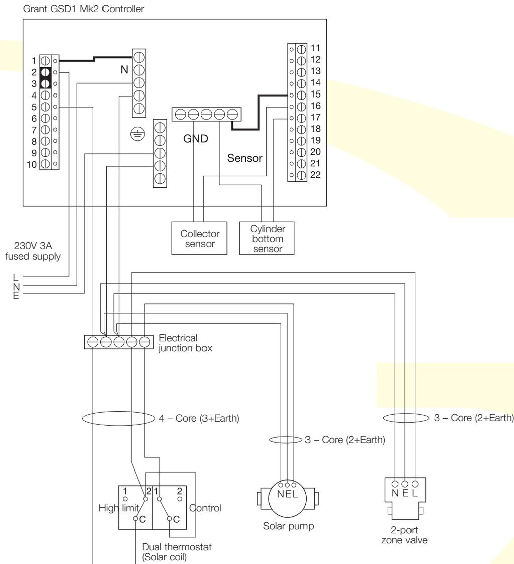
**Figure 5-4:** Cabling diagram for system controls
