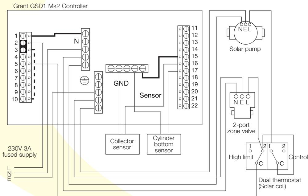
Figure 5-3: Solar thermal system wiring diagram
