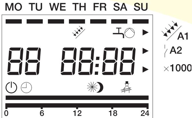
Figure 3-3: Controller display
