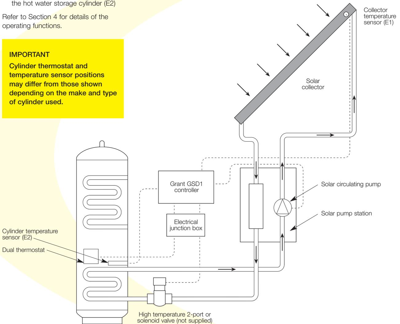
Figure 6-1: Schematic diagram of Grant solar thermal system
