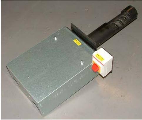
Figure 3-4. Auger unit with cover fitted
