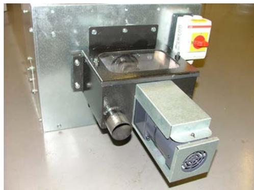
Figure 4-8. Auger unit mounted on store
