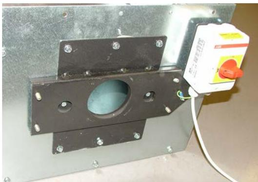
Figure 4-7. Auger unit mounting flange fitted
