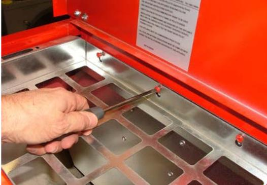
**Figure 4-17.** Secure dam plate and grille
