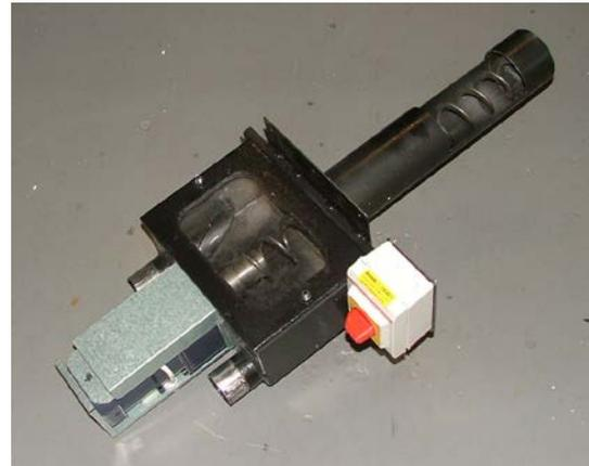
Figure 4-2. Auger unit with cover removed
