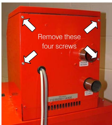
Figure 7-1. Cover fixing screws - rear
