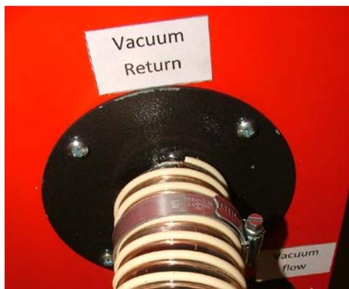
**Figure 4-22.** Tube secured with clip
