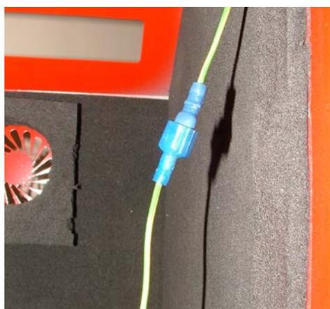
Figure 7-3. Earth wire connector
