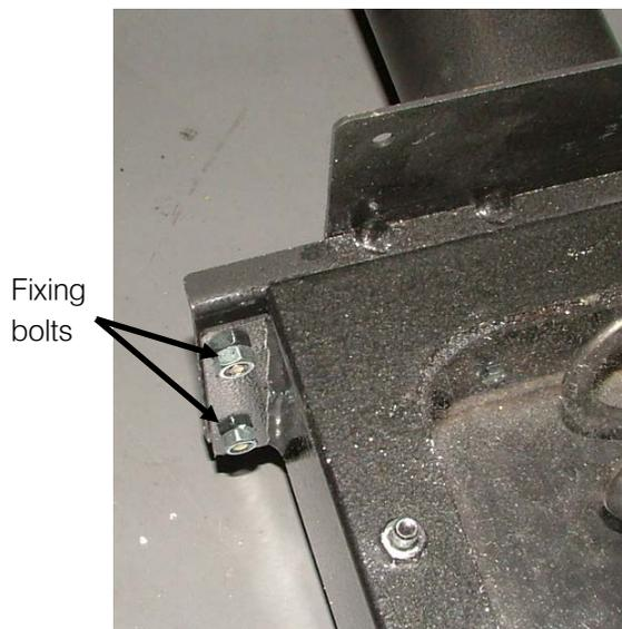
Figure 4-3. Auger unit flange fixings - left
