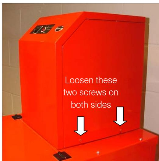
Figure 7-2. Cover fixing screws - sides
