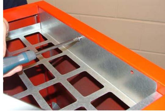
**Figure 4-18.** Fix grille at front edge
