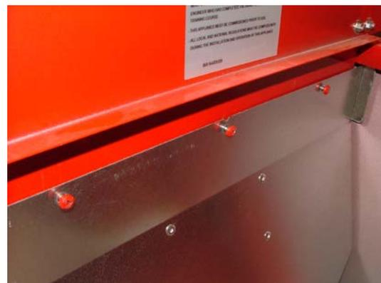
Figure 4-16. Pellet dam plate fixings
