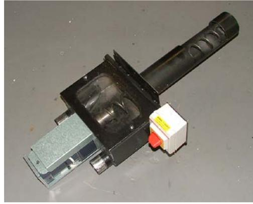
Figure 3-5. Auger unit with cover removed
