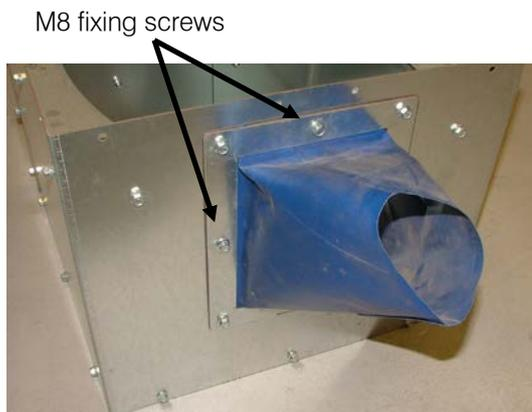
Figure 4-5. Bulk store flange/auger sleeve
